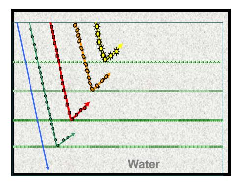
Micro Filtration (MF) (10-0.1μm) Bacteria, suspended particles
