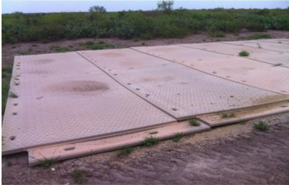
Figure 53. A second use of the Newpark mats was for a pad for field trials. The pad must be secure for equipment as well as preventing punctures of containment during tests. Note panels are not locked together due to a shortage of lock/pins.
